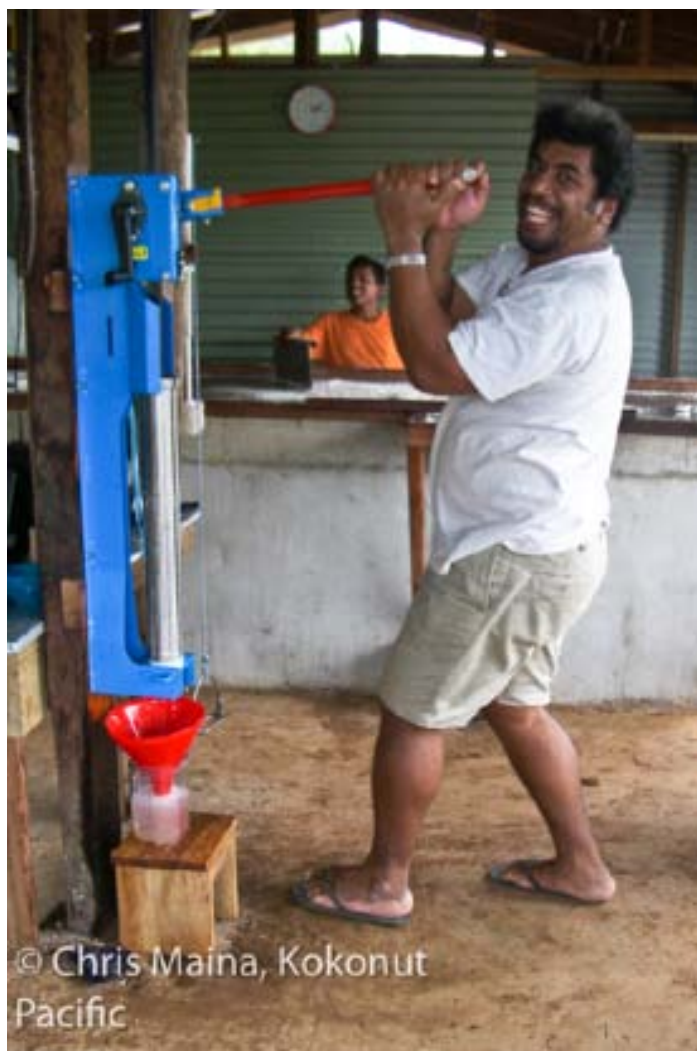
Top: Shredding coconut kernel using simple motor-driven graters. Bottom: Lever-operated Direct Micro Expelling press. Both photos: Fiji.
